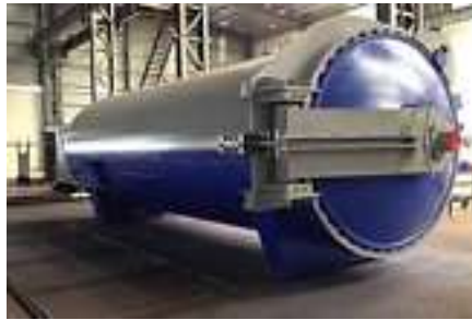
Fig. 1. Autoclave used in the vulcanization process
